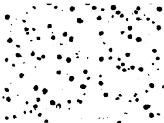
Figure 2 Sketch of spheroidal graphite in cast iron.
