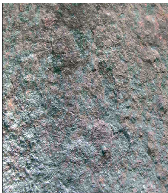
Figure 9 Surface condition of a lamellar graphite iron casting exposed for several decades to atmospheric corrosion. Reproduced with permission from Reynaud, A. Corrosion and Cast Iron , ETIF, France, 2008.
