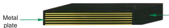
Figure 6 Rubber-to-metal bonding products – (a) tank lining (LHS), (b) various automotive rubber products (RHS) and (c) below rubber bridge bearing.
