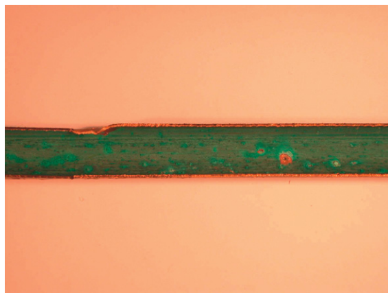
Figure 3 Photograph showing carbon film pitting on a copper tube.
