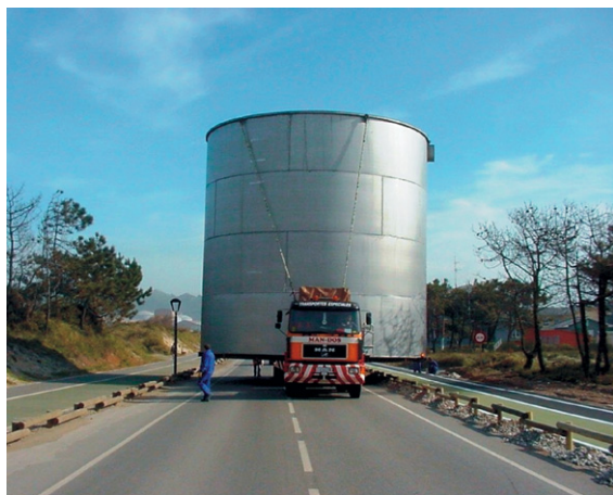
Figure 50 A tank on the road in stainless steel grade S2750 (1.4410).
