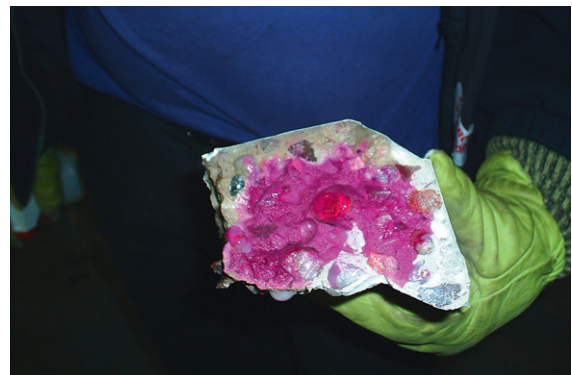
Figure 4 Carbonated concrete sample treated with phenolphthalein indicator (magenta color represents uncarbonated concrete).
