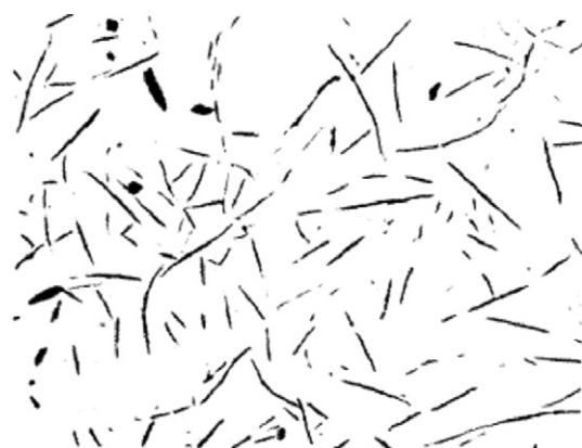
Figure 1 Sketch of lamellar (flake) graphite in cast iron.
